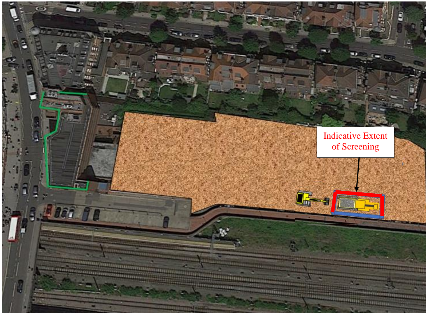
FIGURE 3 – PROPOSED SITE SET UP FOR CRUSHING PLANT
